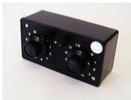
Figure 10 - 0 to 10-ohm Track Circuit Test Shunt Box
