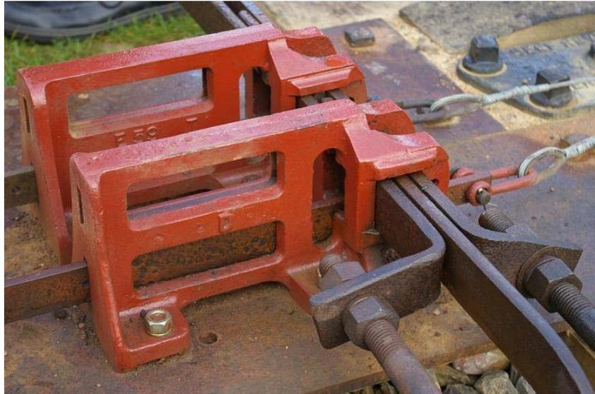
Figure 5 - Mechanical Detector
