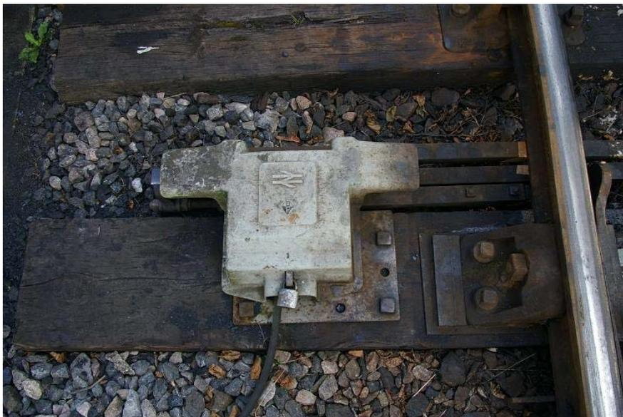
Figure 6 - BR Standard Electrical Detector
