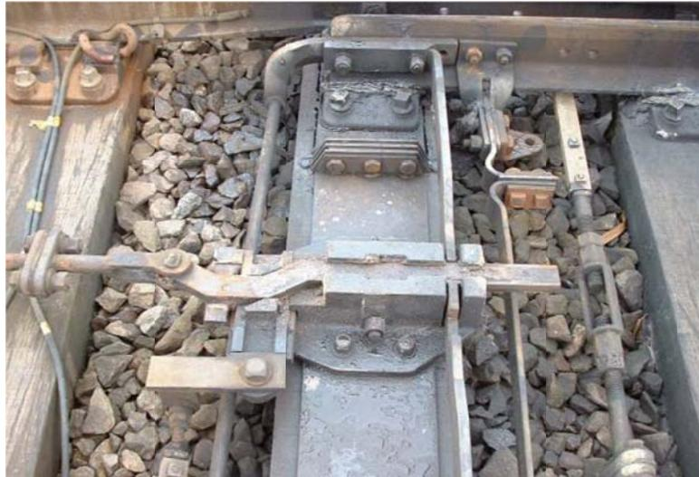
Figure 2 - Standard Facing Point Lock
